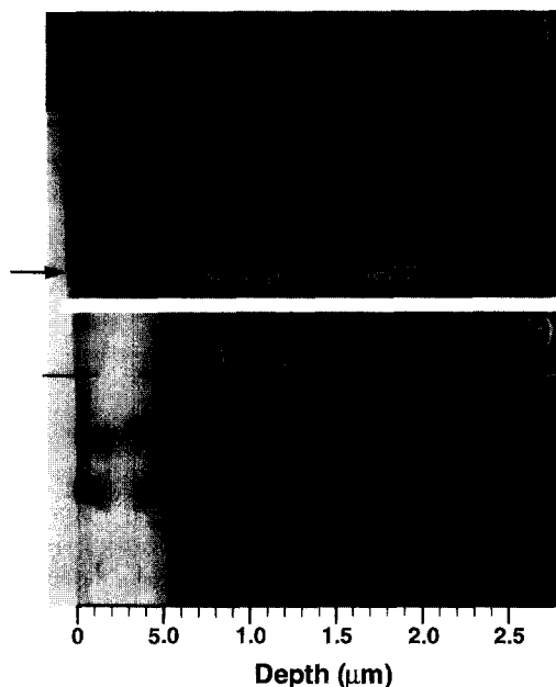
Fig. 9. XTEM images of samples irradiated with 360 keV \text{Ar}^{2+} to (a) 8 ions/ \text{nm}^2 at 170 K and (b) 20 ions/ \text{nm}^2 at 370 K.
